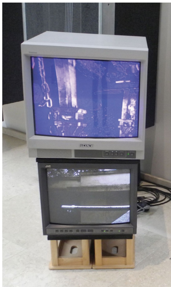
Figure 4 Shifted colour temperature on one of the CRT monitors in Das Deutschlandgerät . (Photo: Documentation archive of the Conservation Department, Kunstsammlung Nordrhein-Westfalen, 2019.)
