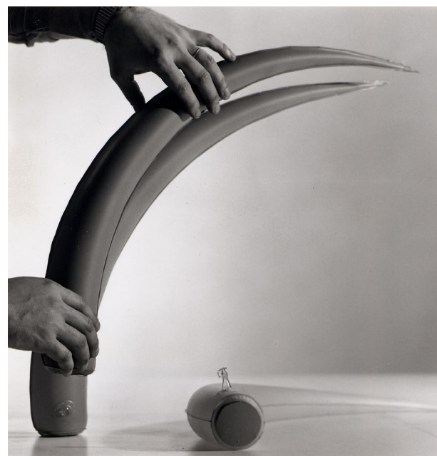
Figure 1 Part of the P-PVC model of the EURODOUMS 4 pressostatic and self-standing dome (Turin, 1972) realised in collaboration with Plasteco (Milan). Original photograph by DDL studio, now part of the CASVA archive. (Photo: Comune di Milano/CASVA.)
